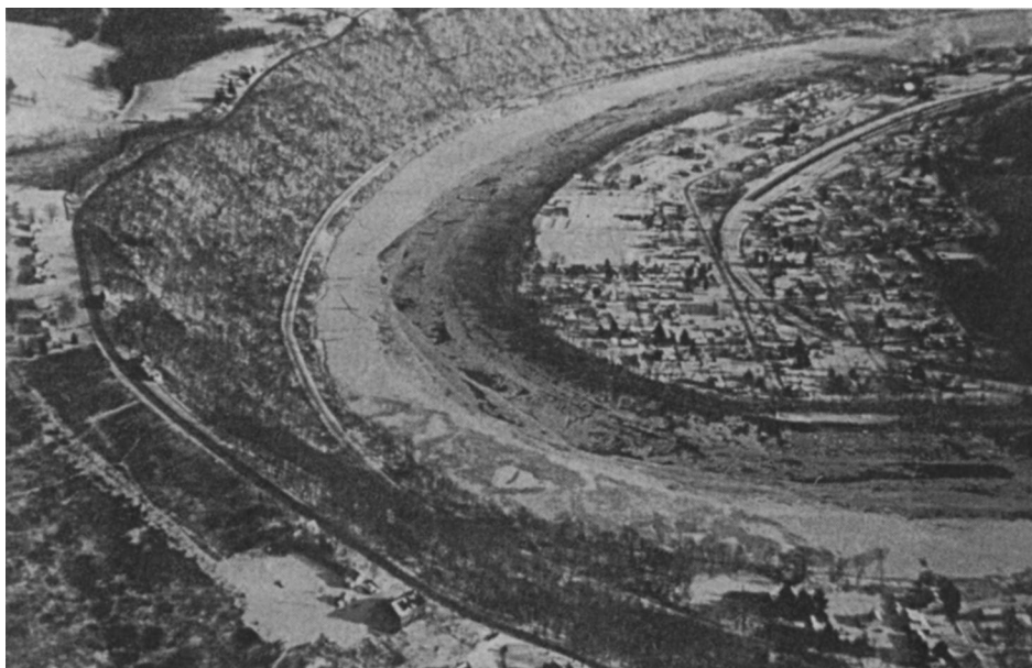
Figure 3-11. Broken, irregular vessel track around a sharp river bend, indicating difficulties in navigating through the ice.
